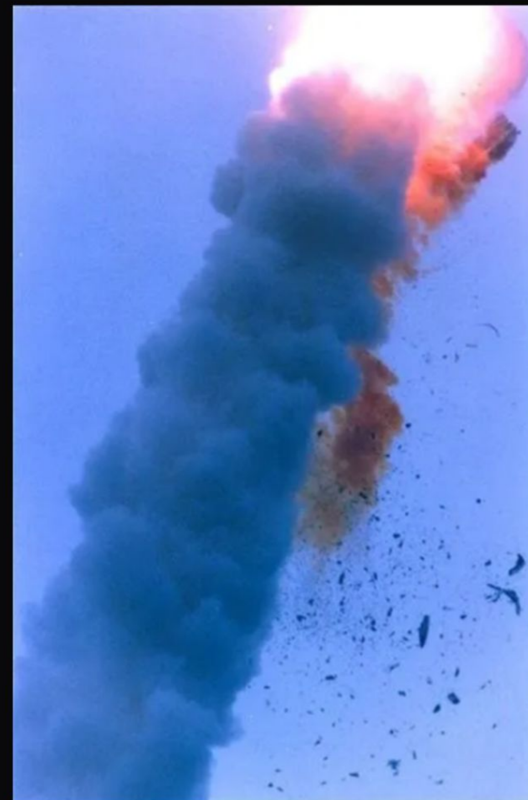
Ariane flight V88 exploded on 4 June 1996 because of inadequate overflow protection
